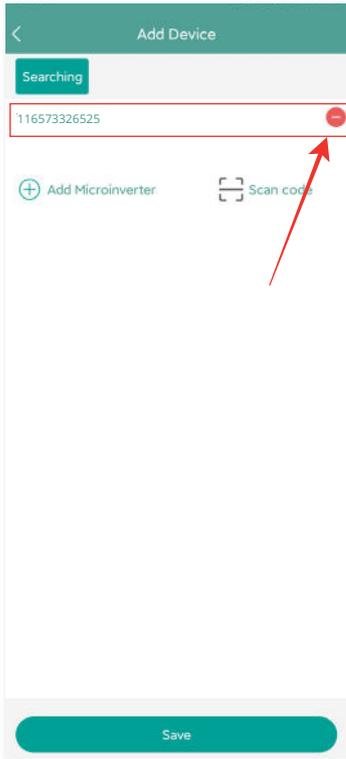
5. Confirm that the microinverter ID in the list is correct, and tap Save.
