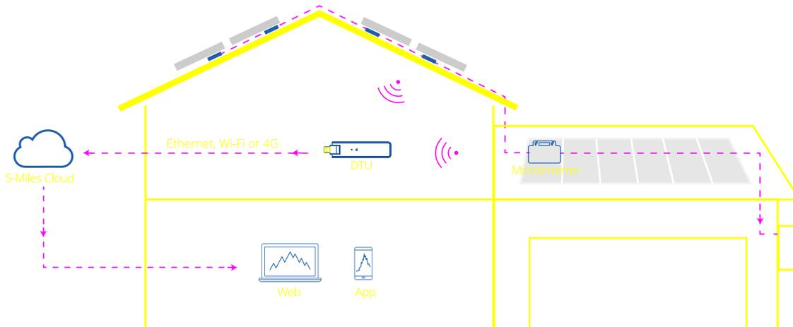
The complete Hoymiles PV microinverter system is composed of PV microinverter, Hoymiles gateway DTU and Hoymiles S-Miles Cloud.
